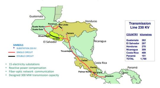
The Central America Operational Planning 2023-2024<sup>7</sup> contemplates the entry between January 2023 and December 2024 of 27 projects for a total of 1,660.8 MW of new capacity in the countries of the region. Of the total, 25 projects for nearly 500 MW are renewable and are expected to be added to the system in the 2023-2024 period. The document includes four projects in Nicaragua,
